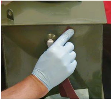
Sand or brush repair area
